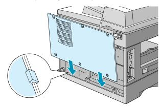
**12** Slide the cover to the right and align the connectors on top of the cover with those on the machine. Fasten the six screws to secure the cover.
